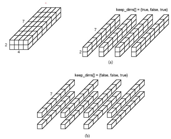
Splitting a Cartesian topology of size 2 x 4 x 7 into (a) four subgroups of size 2 x 1 x 7, and (b) eight subgroups of size 1 x 1 x 7.
