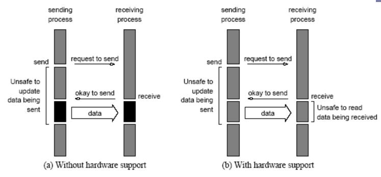
Non-blocking non-buffered send and receive operations (a) in absence of communication hardware; (b) in presence of communication hardware.
