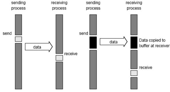
Blocking buffered transfer protocols: (a) in the presence of communication hardware with buffers at send and receive ends; and (b) in the absence of communication hardware, sender interrupts receiver and deposits data in buffer at receiver end.
