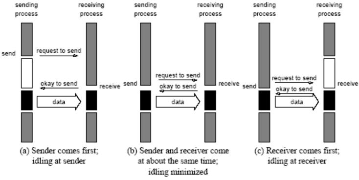
Handshake for a blocking non-buffered send/receive operation.
