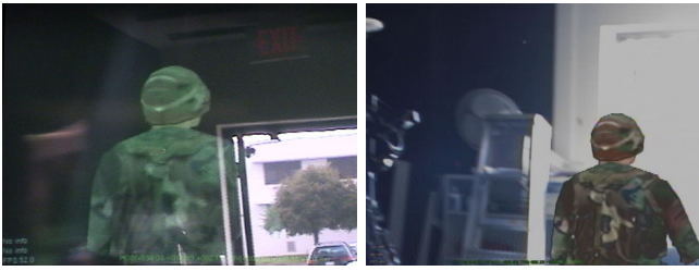
Figure 3: Left: Optical see-through leaves synthetic objects with a ghostly appearance. Right: Graphical overlay on video enables full occlusion of real objects by synthetic objects.
