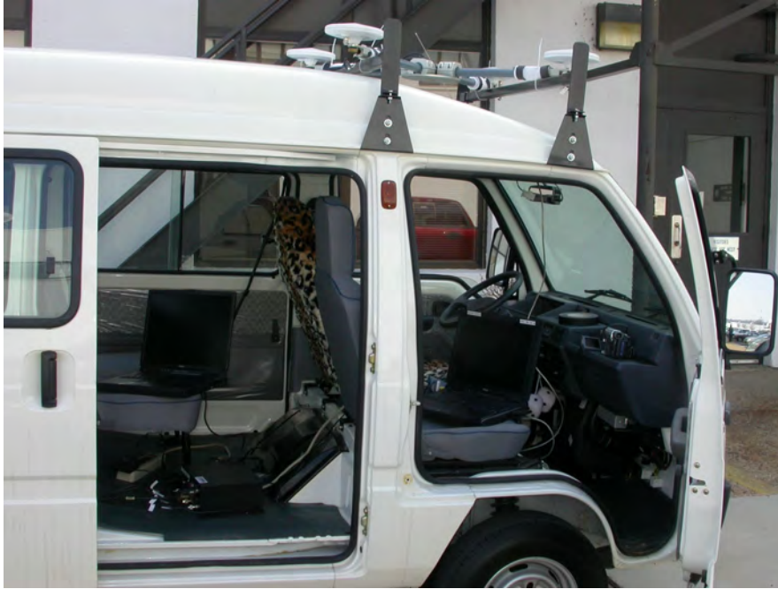
Fig. 3 An early prototype for a vehicle-mounted system included a four-antenna GPS unit on the roof for position and orientation and mobile computers inside for computation and display.
