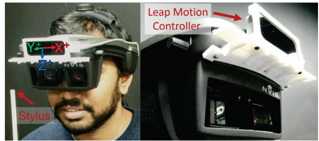
Figure 2: (right) Our HMD and Leap Motion system. (left) A user performing stylus to screen alignments. The right-handed head relative coordinate frame, in relation to the Leap Motion, is shown. Positive X extends horizontally to the user’s left, positive Y forward, and positive Z downward to the ground.
