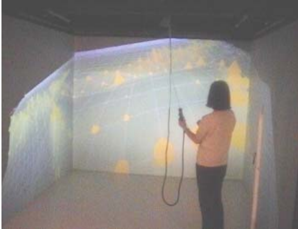
Fig. 3: Shows a test application driving a CAVE using the pc commodity cluster.
