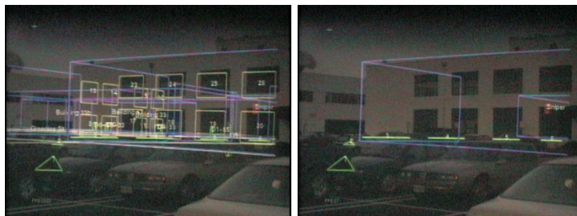
Fig. 3 The need for information filtering. Left: "raw" data, a confusing clutter of many different labels and objects. Right: filtered output draws the foreground building for context, the path the user is following, and a potential threat.
