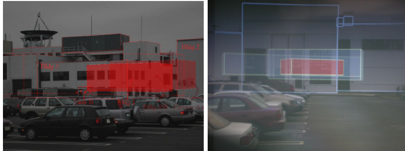
Fig. 7: Left : one of the concept sketches for how occluded buildings and units might be represented in BARS. Right : a photograph taken through our optical see-through display with a similar protocol implemented.
